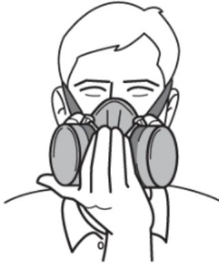
**Seal checks for disposable respirators:** A seal check can be done by placing both hands over the respirator itself, or by using a device provided by the manufacturer.
