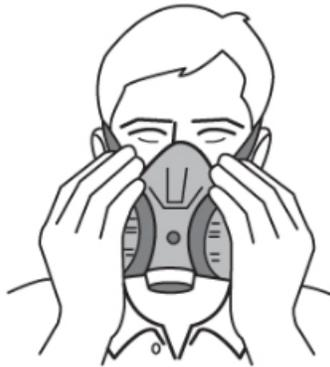
**Positive pressure seal check:** Positive-pressure seal checks can be done with respirators equipped with tight-fitting facepieces that have both inhalation and exhalation valves.
