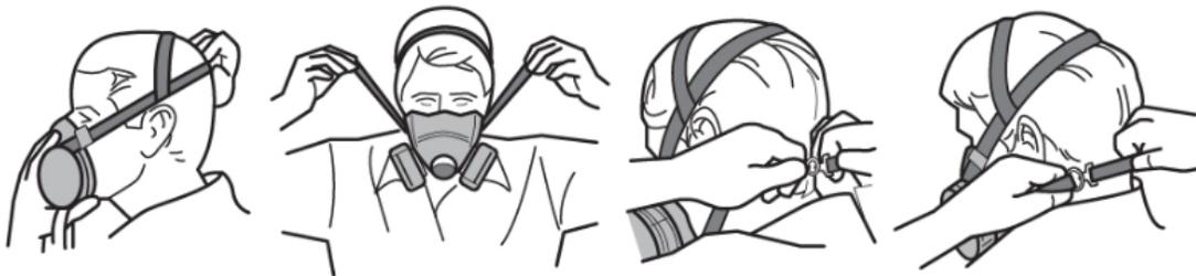
Elastomeric facepieces are made of silicone, thermoplastic, or rubber material. One or more filters or cartridges are attached to the facepiece.
